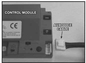
Figure 12.9 AUX 300 module installation
